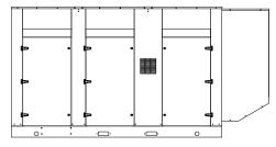
"LEVEL 2" HOUSED GEN-SET Full aluminum weather protection and superior sound attenuation for specific low noise applications. <u>Critical grade muffler is standard.</u>
